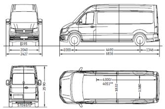
Illustration shown is CR35 long wheelbase panel van with high roof.
